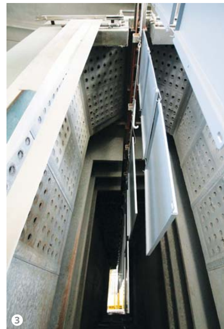
Figure 3: Workpieces entering the 5-stage pre-treatment tunnel.
