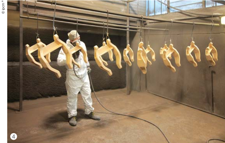
Figure 4: The liquid application stage in the static booth.
