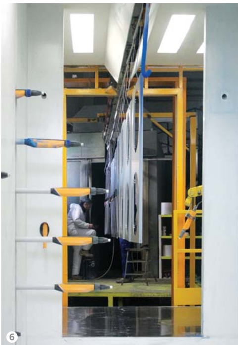
Figure 6: The dynamic reciprocator in function.
