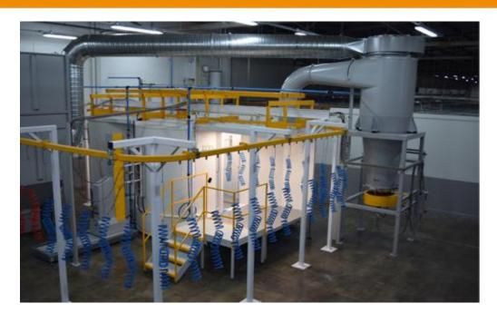
With a diverse range of colours, the need for fast colour change and criticalness of the powder consistency across the entire spring the Magic Cylinder booth, coupled with the OptiCentre and latest generation application guns provided the perfect solution to Hanson Springs. Many of the part geometries in associated with spring coating
