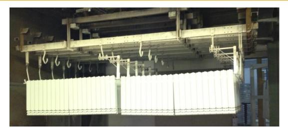
Quality Increase: the new automatic guns coat perfectly the whole surface of the radiators even in cavities and in less visible areas. Color change: 90% of the production is coated by two different types of white. There is an increasing demand for special colors. Thanks to the Gema solution, using the EquiFlow concept and OptiCenter, Faral has the best condition for each situation.
