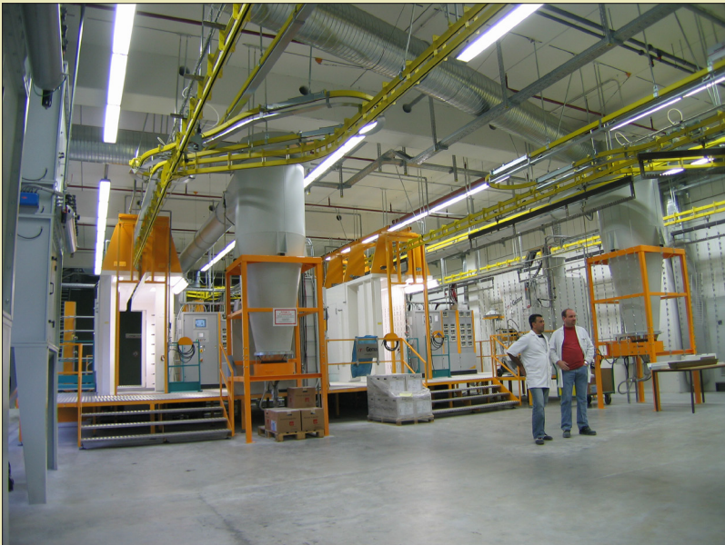
(top) The powder coating line has been separated from the loading area.
