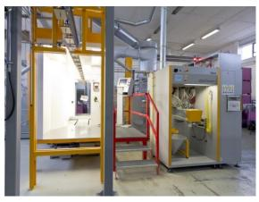
the engine blocks. A fully automatic coating process was initially unthinkable to the Sarnoch specialists. However, tests at the Gema lab in St. Gallen could convince them of the contrary: OptiGun powder guns impressed with their high penetration and provided perfect results.
