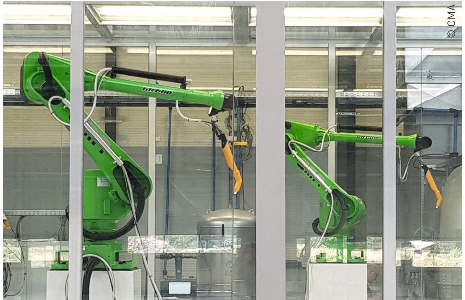
Figure 25: CMA Robots for Powder Coating
