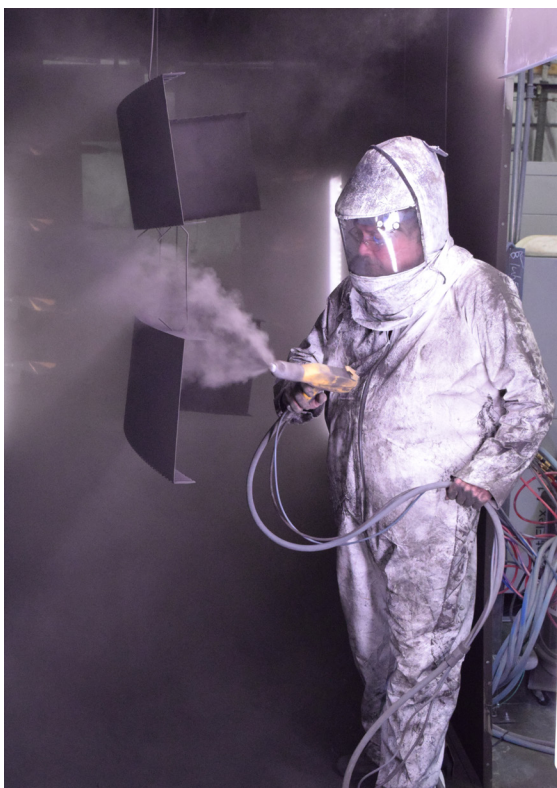
Figure 3 Manual operators performed well but needed ample room to apply the powder coating. The company sought to increase line density to improve productivity.
